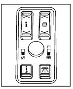
The HUD controls are located to the left of the steering wheel on the DIC control panel.
